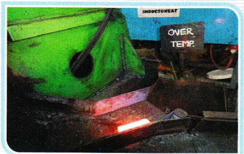
We have hot shearing facility through induction long bar heaters. We carry out quality inspection like dimension, weight and visual inspection of cut blanks. Also both shearing machines are equipped with GO – NO GO System for controlling Over Heated and Under Heated cut pieces.
